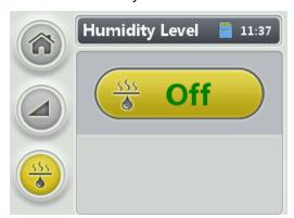
Rotate the control wheel to the **Humidity Level** menu and press the control wheel to enter the **Humidity Level** screen.
