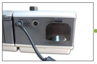
Connect the DC power plug of the power adapter to the DC power interface on the back of the ventilator and connect the AC power plug to the AC power socket.
