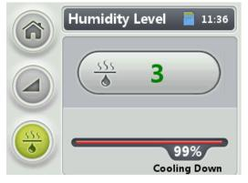
3. (When Humidity Level is not set to Off) Before treatment, press and held the control wheel for 3s. If the ventilator is not in Warming Up or Cooling Down state, the temperature and humidity levels of the humidifier are increased. If the ventilator is in Warming Up state, the temperature and humidity levels are reduced.
