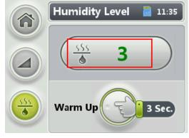
Rotate the control wheel to select a humidity level and press the control wheel to confirm the selection
